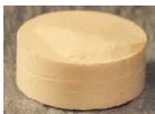
Delamination (cracks along band)
